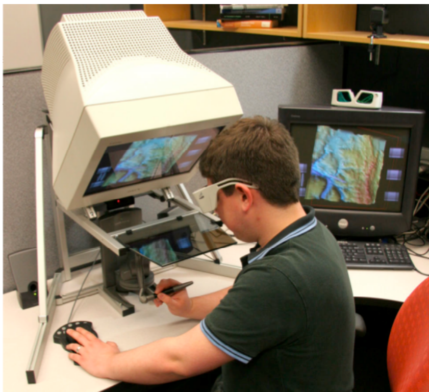
Figure 13. Using a collocated setup where active stereo graphics are displayed onto a mirror, beneath which the Phantom is operated
