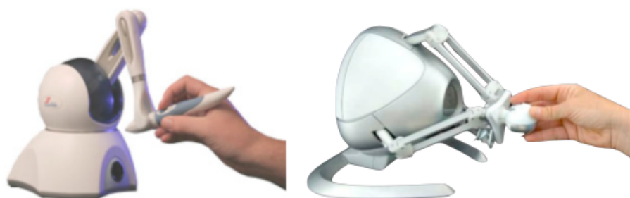
Figure 12. Low-end point force feedback devices: Phantom Omni (left) and Novint's Falcon (right)
