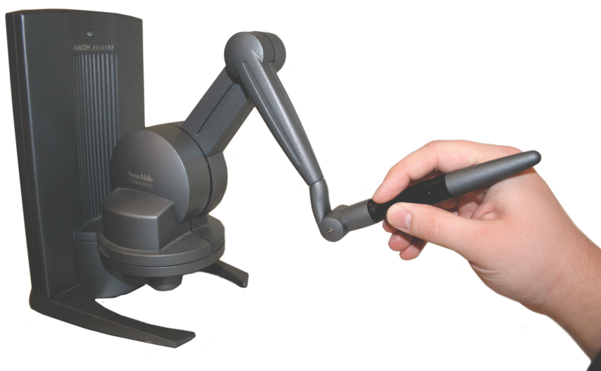
Figure 25. Phantom haptic force feedback device
